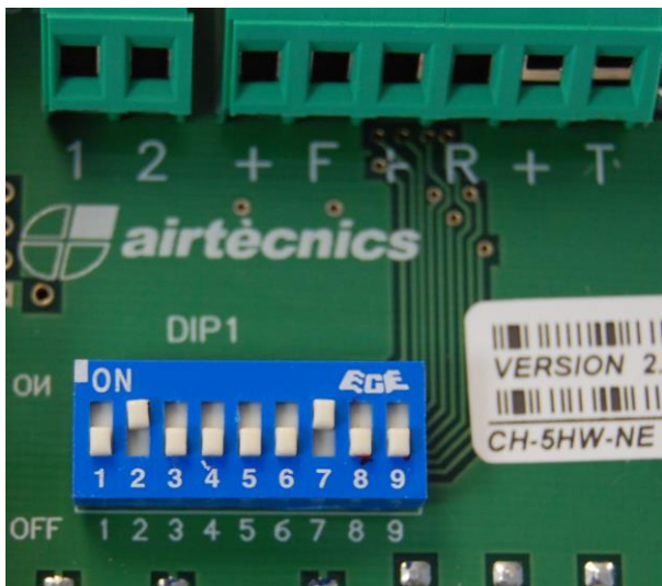
2 and 7 position ON – With magnetical/mechanical door contact
