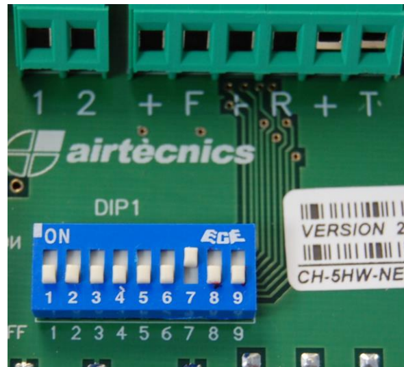
7 position ON – Without magnetical/mechanical door contact
